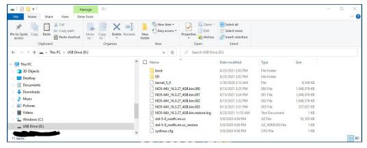
The example below is a compressed image that was backed up via the 10ZiG Manager and then copied to the thumb drive for purposes of restoring the image.
