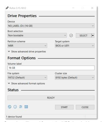
Open the utility and format the USB thumb drive as "Non bootable", and FAT32 and then run the utility on the USB thumb drive.
